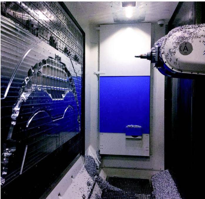
Bulkhead - Alluminum 7040 966 x 1347 x 178 mm - 38.5 x 53 x 7" 400 Kg > 7,5 Kg in 6- hours
