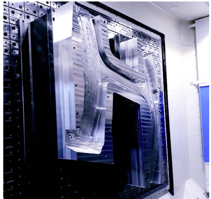
Windshield - Alluminum 7475 2540 x 1067 x 50 mm - 100 x 42 x 2" 700 Kg > 12 Kg in 20- hours
