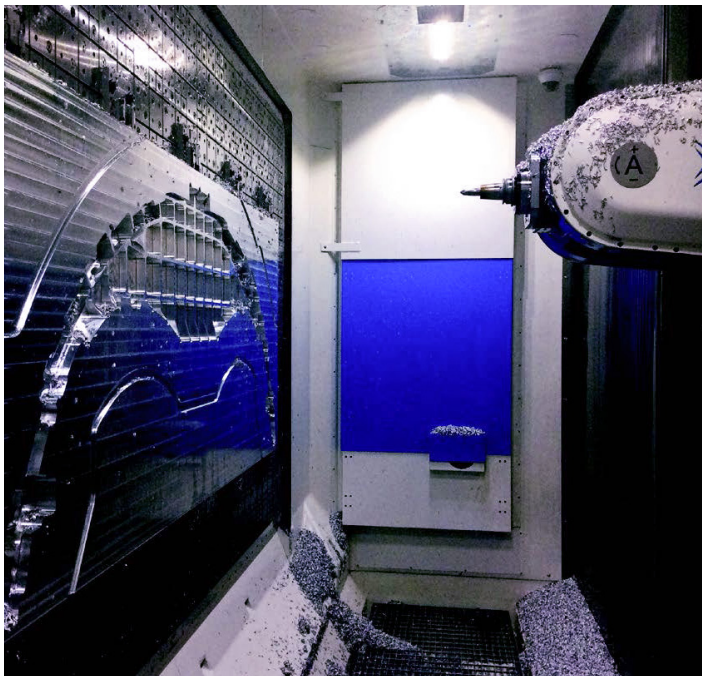
Bulkhead - 舱壁-铝 7040 966 x 1347 x 178 mm – 38.5 x 53 x 7” 400 Kg > 7,5 Kg in 6- hours
