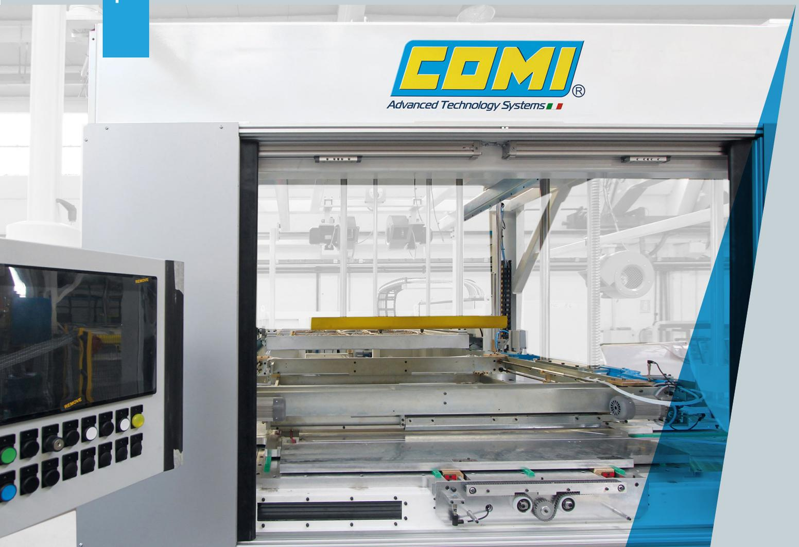
The LaborForma serie's thermoforming machines are suitable for working plastic materials HIPS / ABS / PMMA / PP in cycle, with thickness up to 12 mm.
